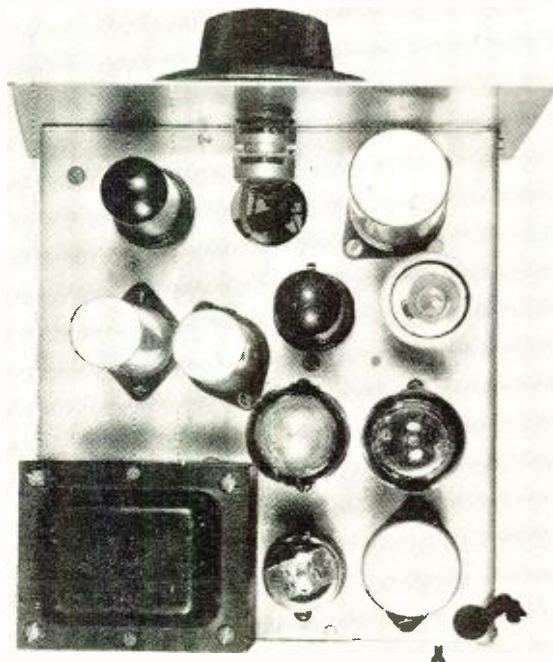
Fig. 5. Top chassis view of unit. The line "on-off" switch, S 2 , is mounted on rear flange of chassis, lower right in photo.
