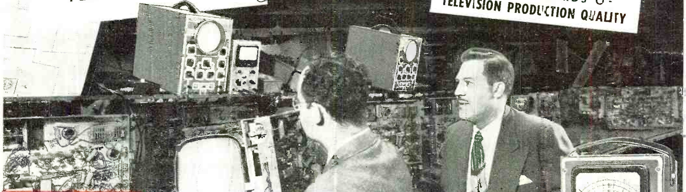
Tele-King Production Test Foreman James Adler and Harry R. Ashley, President of EICO, inspecting the use of the EICO Model 425 Oscilloscope and Model 221 Vacuum Tube Voltmeter at one of the important constant alignment positions on the Tele-King television production line, New York City.
